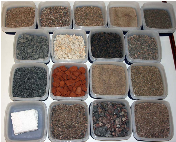
Fig. 3. Samples. (Top row) Play, Safety, Concrete, Filler, and Golf (Lohja Rudus sand). (Second row) Diabase, Quartz, LECA, and (sanding) Gravel. (Third row) Gabbro, Crushed Brick, Sand 0.1–0.6 mm, and Sand 0.5–1.2 mm (commercial samples). (Lowest) Polystyrene and natural targets: Beach and Harbor sand and gravel, and Bunker sand.
