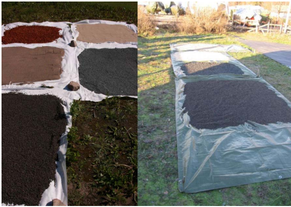
Fig. 8. (Left) Calibration gravel samples set up for the Nuuksio July 2007 ALS campaign. (Clockwise from top left) Crushed redbrick (C Brick), sandblasting sand (Sand01), black gabbro (Gabbro), crushed LECA (LECA), and sandblasting sand (Sand05). (Right) The gravel samples at the Espoonlahti December 2007 campaign. (From top downward) Gravel, Quartz, Diabase, and LECA.
